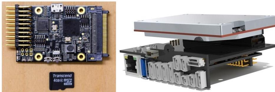
**Figure 6. Prioria's Merlin Autopilot hardware design. A Merlin flight controller is seen on the left and a rendering of the Merlin flight controller with vision computer is seen on the right.**
